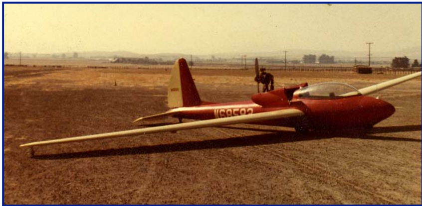
Photo showing the engine doors open prior to retracting the engine. Doors are closed when the engine is extended or retracted
