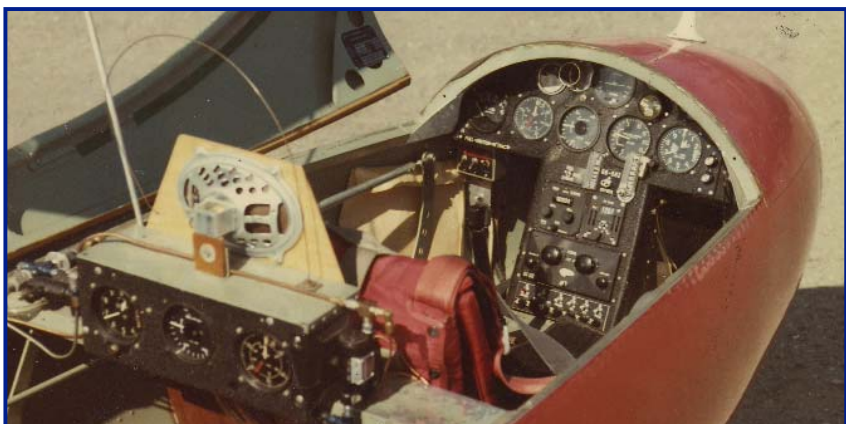
Aircraft has fully equipped instrumentation and avionics equipment. Also oxygen equipment for high altitude flying. Even has a altitude reporting transponder.
