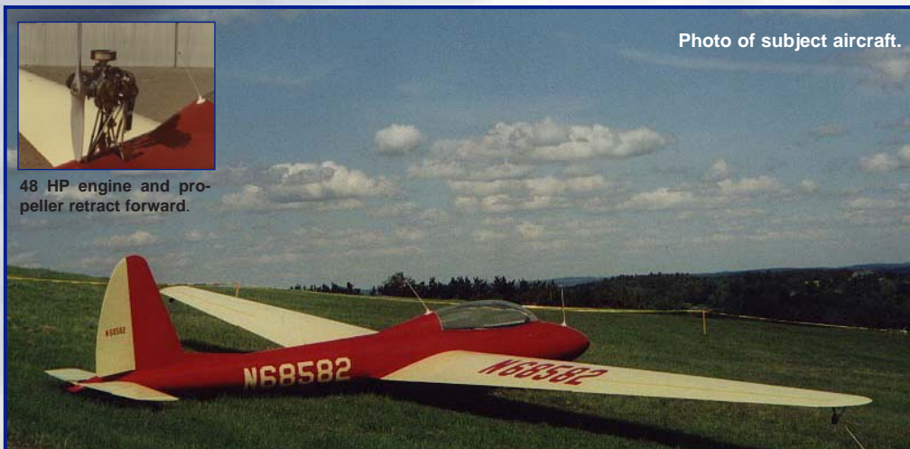
Photo of Ted Nelson's personal Hummingbird. Wingspan 54 feet. The two place all-aluminum aircraft has a glide angle of 27 to 1 which was very good at the time. A Nelson 4-cylinder 2-cycle 48 HP engine produces 350 ft/min climb at a gross weight of 1200 pounds. Takeoff distance is about 700 feet at a climb speed of 58 MPH. Six were manufactured.
